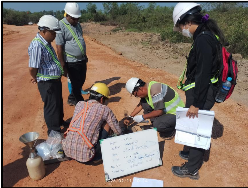
Item : Field Density Test Description : CR2-16,CR2-2,MA2-1(L) Date Taken : February 11, 2026
