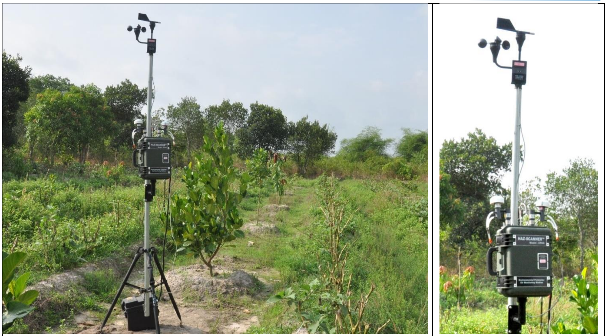
Figure 4. 28: Air Quality Measurement Device
