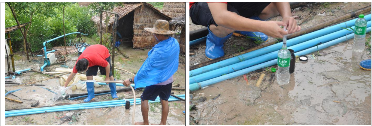
Ground water sampling at farmhouse which lies near proposed wastewater treatment plant
